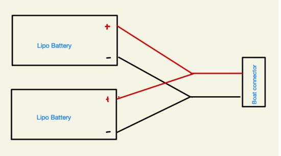
Figure B-2: Battery connection [13]
