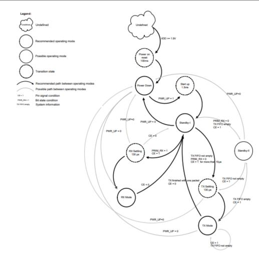
Figure C-3: State Machine for Transmission System [16]
